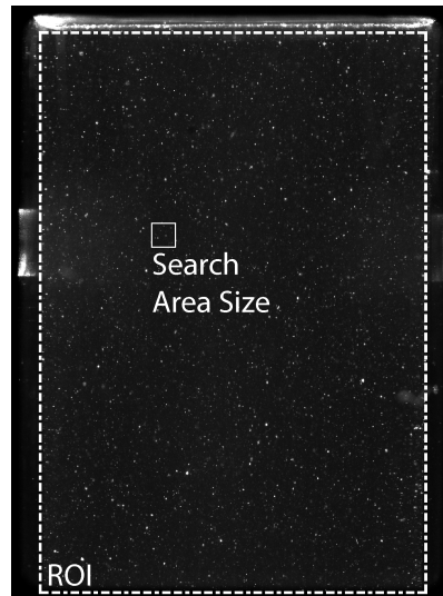
Figure 5.17. Photograph of a seeded flow in the transparent mixing chamber with the indication of the ROI and the search area size.
