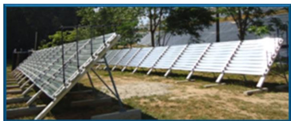
Figure 9.27. Semi-industrial plant for the treatment of 20 m 3 /day of leachate, developed under the project Advanced LFT.
