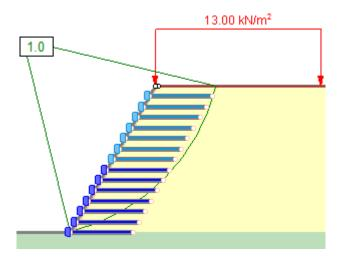
Figure 8. Global Minimum slip surface and over-design factor of Slope 7 ( $\alpha$  = 60°, L = 3.6 m,
