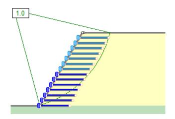
Figure 5. Global Minimum slip surface and over-design factor of Slope 4 ( $\alpha$  = 60°, L = 3.4 m,
