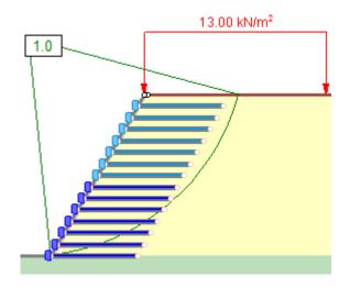
Figure 7. Global Minimum slip surface and over-design factor of Slope 6 ( $\alpha$  = 60°, L = 4.5 m,
