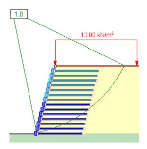
Figure 10. Global Minimum slip surface and over-design factor of Slope 9 ( $\alpha$  = 75°,
