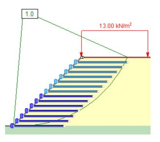
Figure 9. Global Minimum slip surface and over-design factor of Slope 8 ( $\alpha$  = 45°, L = 6.3 m,
