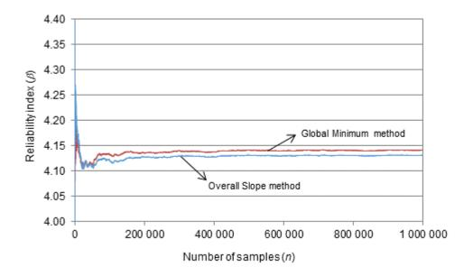
Figure 11. Convergence of the reliability index of Slope 5 (Global Minimum and Overall Slope
