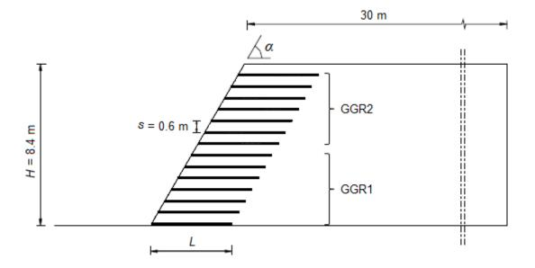
Figure 1. Schematic illustration of the geosynthetic-reinforced slopes
