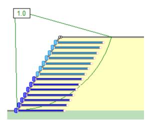
Figure 3. Global Minimum slip surface and over-design factor of Slope 2 ( $\alpha$  = 60°, L = 5.4 m,
