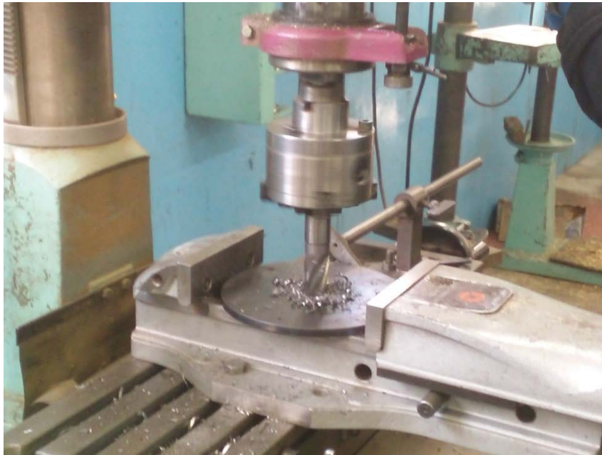
Figure 2.14: Drilling brass plate to fix at “Castro Lighting” factory.
