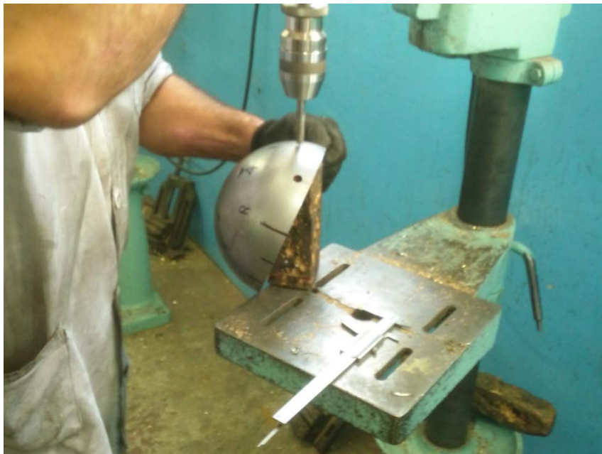
Figure 2.16: Drilling brass plate to fix at “Castro Lighting” factory.
