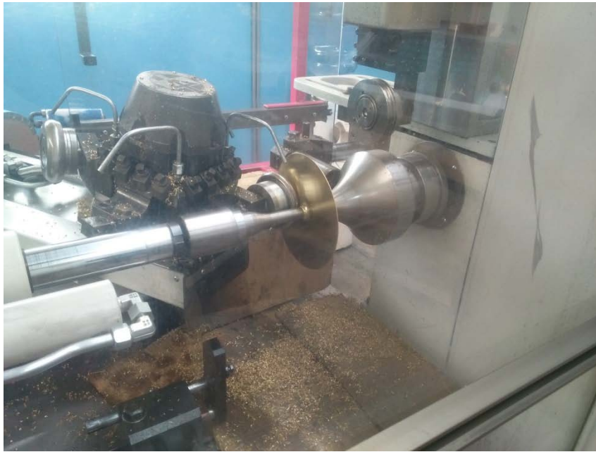
Figure 2.19: Shaping brass plate by machine by metal spinning at “Castro Lighting” factory.
