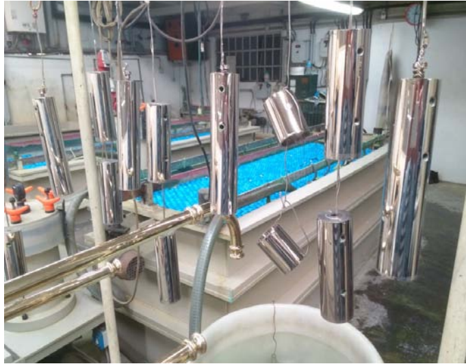
Figure 2.22: Chrome plating brass parts at “Castro Lighting” factory
