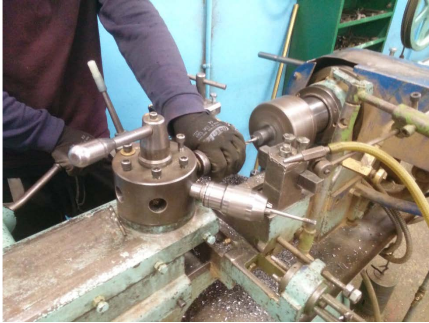
Figure 2.13: Making hole in brass with drill at “Castro Lighting” factory.
