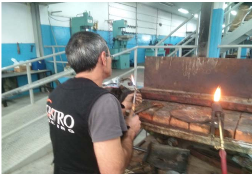
Figure 2.17: Shaping decorative brass pieces by oxy-fuel welding at “Castro Lighting” factory
