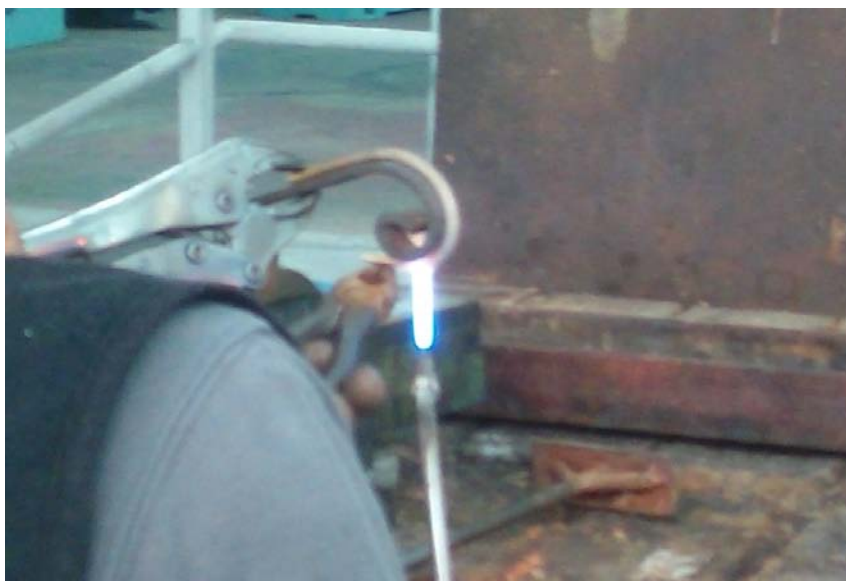
Figure 2.18: Shaping decorative brass pieces by oxy-fuel welding at “Castro Lighting” factory
