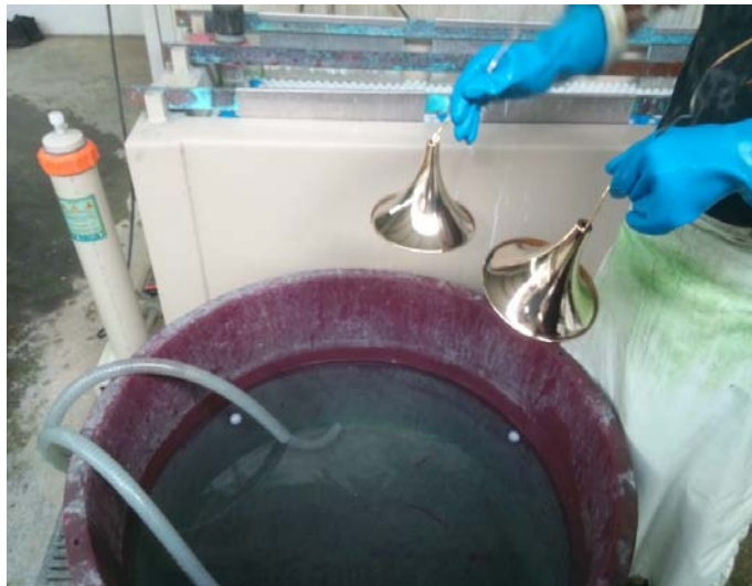
Figure 2.23: Chrome plating brass parts at “Castro Lighting” factory.
