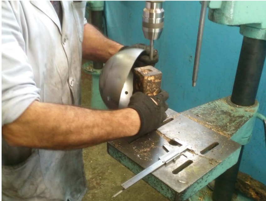
Figure 2.15: Drilling brass plate to fix at “Castro Lighting” factory.
