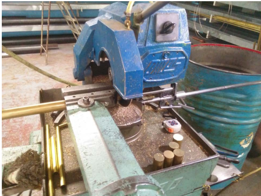
Figure 2.11: Cutting brass tubes by metal cutting saw at “Castro Lighting” factory.
