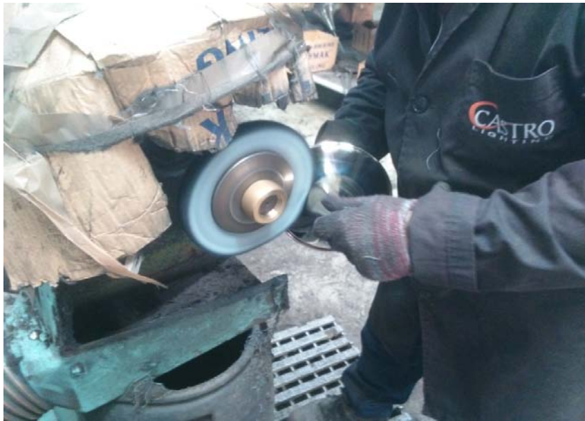
Figure 2.24: Polishing brass basement by polishing machine at “Castro Lighting” factory.
