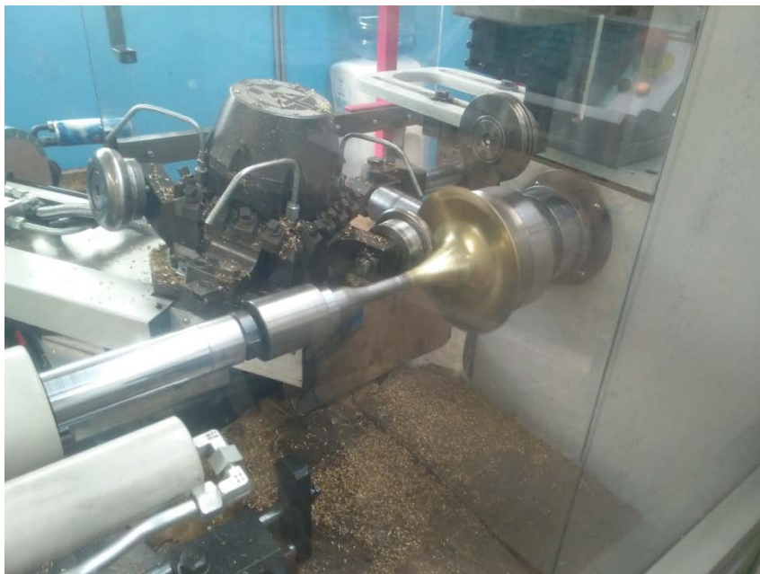
Figure 2.20: Shaping brass plate by machine by metal spinning at “Castro Lighting” factory.
