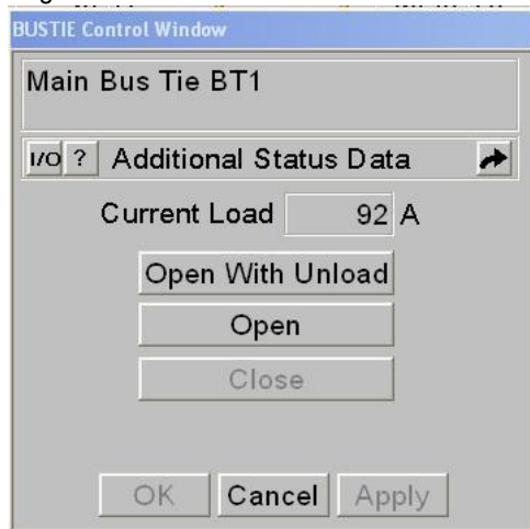
Figure 3.40 – VCS - Circuit Breaker/Bustie Control Window [17].
