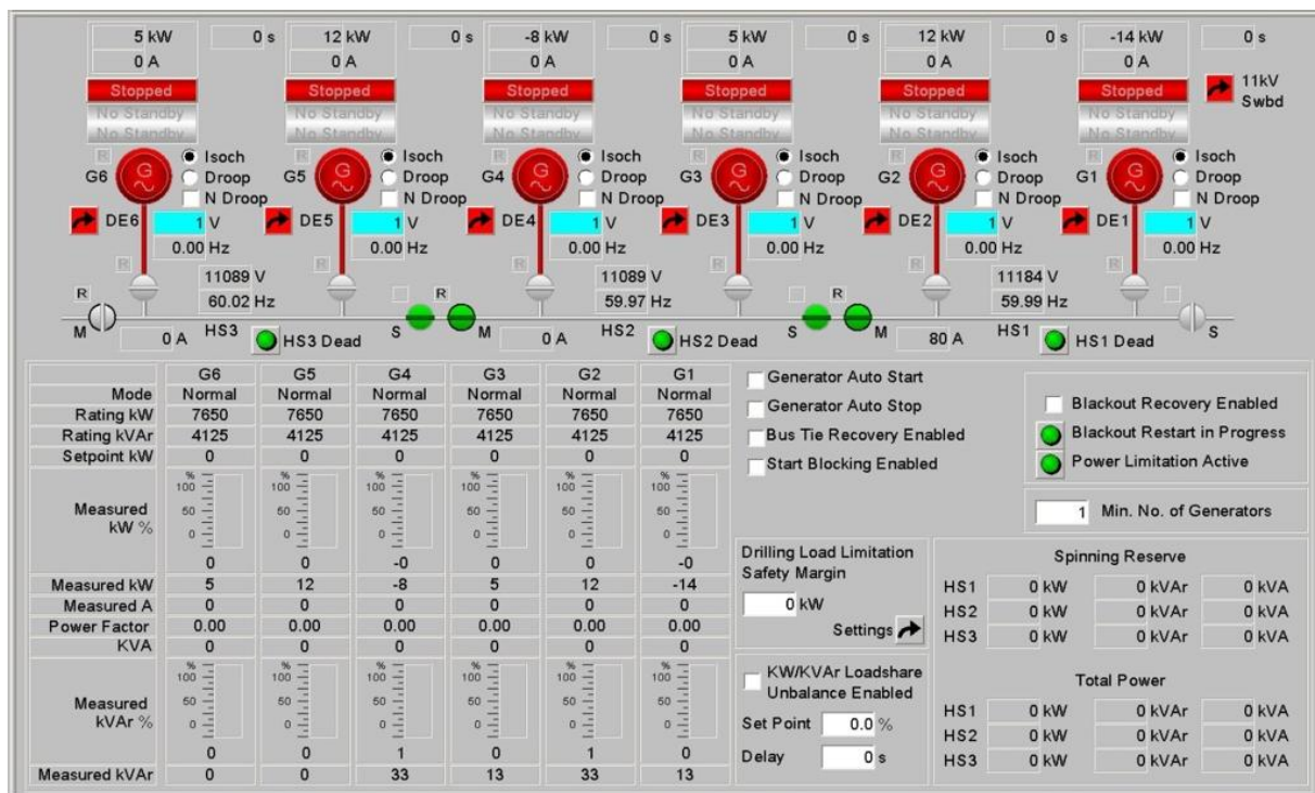
Figure 5.7 – Project - PMS Load &amp; Control HMI [26].
