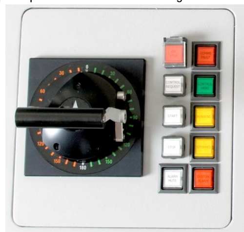
Figure 3.11 – DP - MTC Console Azimuth Thruster Controls [14].
