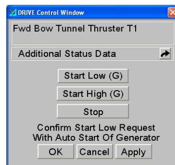
Figure 3.57 – PMS – Drive Control Window [17].
