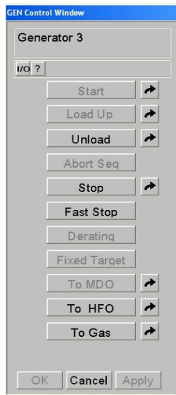
Figure 3.46 – PMS - Generator Control Window [17].
