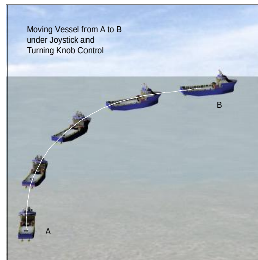
Figure 3.16 – DP - Joystick Manual Heading [14].
