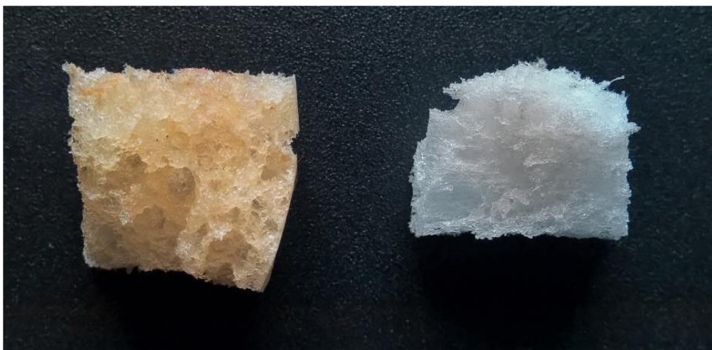
Figure 46: Comparison between populated and pure carrier - PUR A foam after 5 days of operation.
