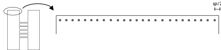
Figure 3.2 - Positioning of particles at the feed channel entrance. The 1 st bacteria, the one on the right, is spaced by sp/2 \mu\text{m} from the channel wall, and the following bacteria are spaced by sp \mu\text{m} . The last bacteria (on the left) is also distanced from the channel wall sp/2 \mu\text{m} .
