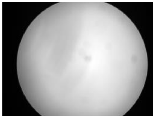
Figure 5.5 Reference averaged image of the illuminated Ulbricht sphere recorded with the infrared camera.
