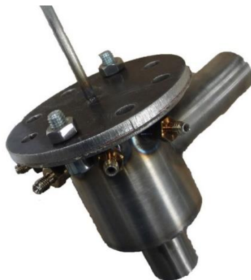
Figure 4.2 Construction of the DE-1 Evaporator
