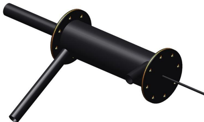
Figure 4.10 CAD illustration of the Evaporator designed for the Diesel evaporation test setup
