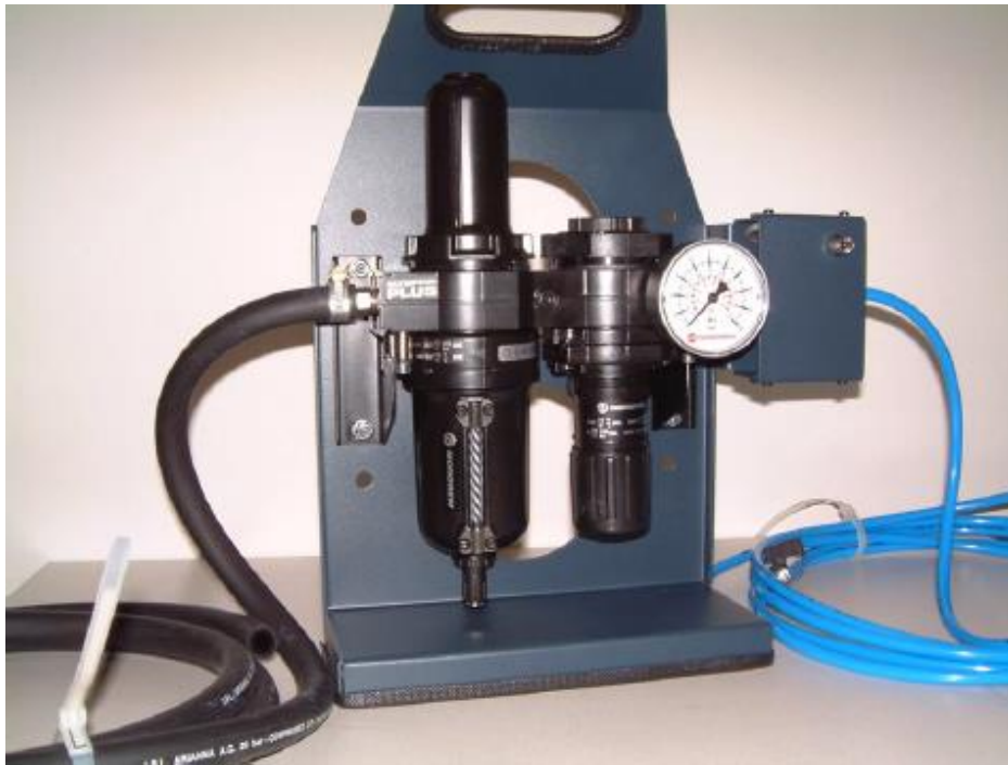
Figure A.4 Unit FU for oil- and dust-free air cooling of the endoscope
