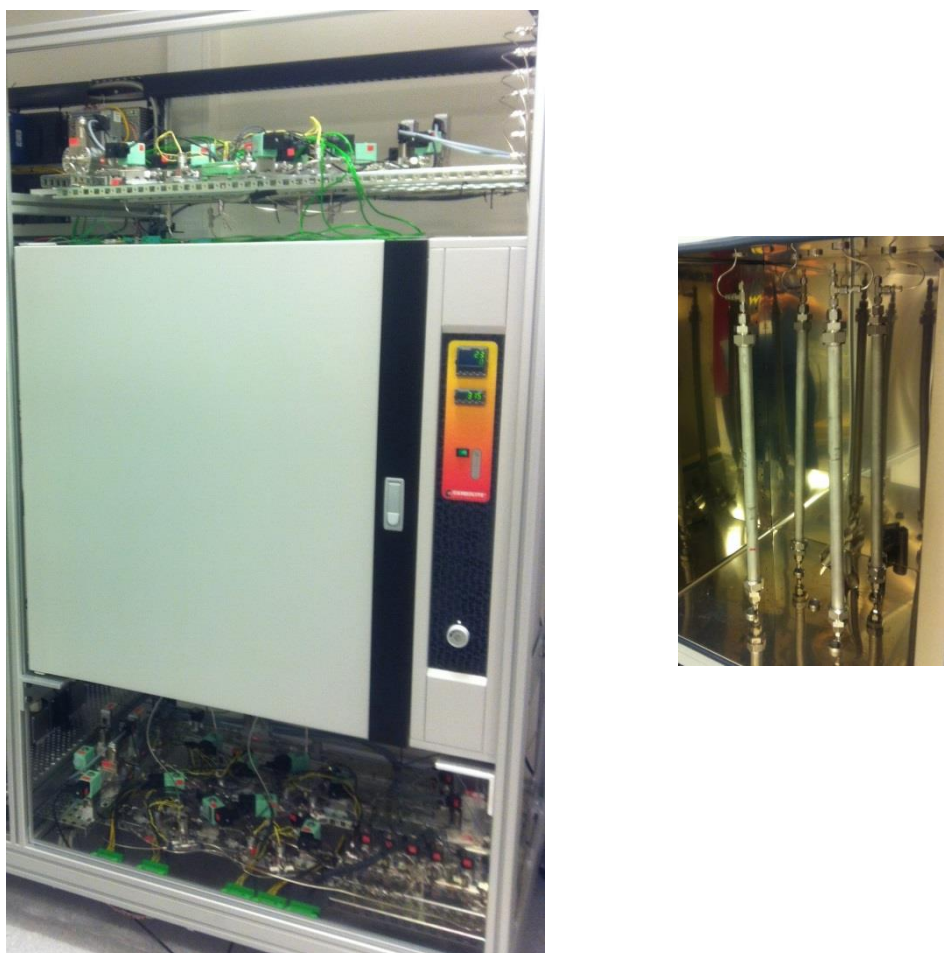
Figure 4.1 - Experimental PSA unit used for the fixed bed experiments
