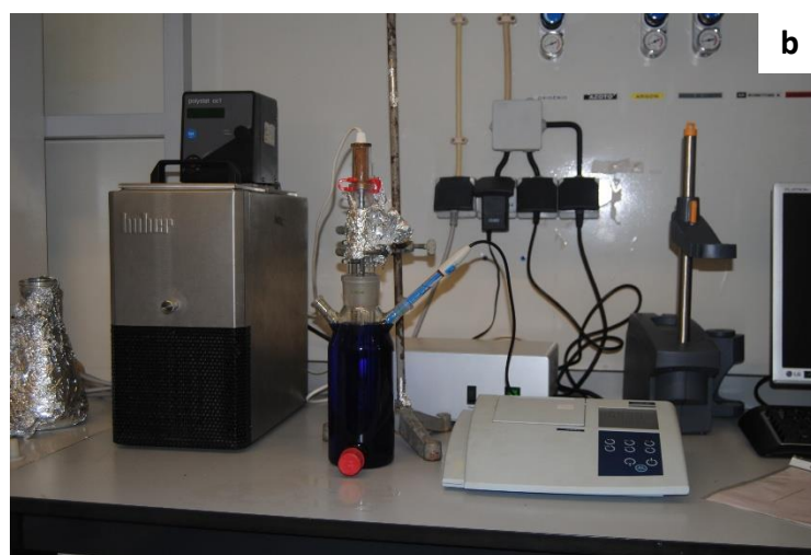
Figure 3.1 - Diagram (a) and photo (b) of the radiation assisted wet peroxidation set-up.
