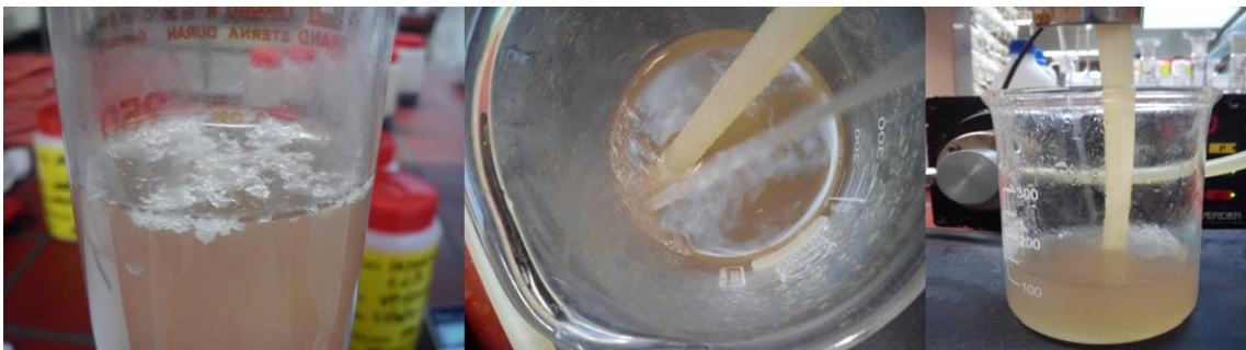
Figure 27 - Results obtained with the fresh starch/0120178.116 solution on the assimilating pump test method.
