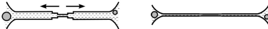
Figure 6 - Stretching of the nodes and transport of the antifoam droplets to the PBs. [4]
