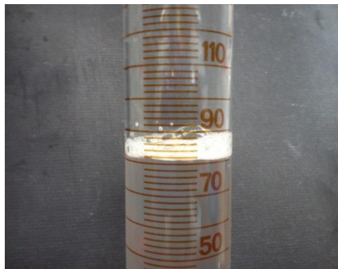
Figure 23 - Residual foam volume of the blank solution after 30 minutes of rest.
