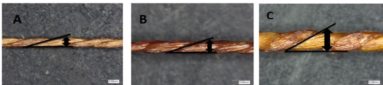
Figure 23 - Microscopic view of Symmetric Hybrids Cords at 550 tpm: ARA220x1+PET238x1 (A), ARA550x1+PET550x1 (B), ARA1100x1+PET1100x1 (C)
