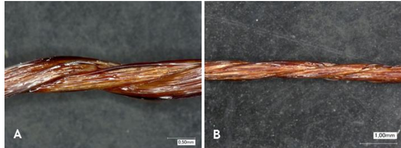
Figure 32 - Microscopic view of ARA1100x1+PET550x1 (A) and ARA550x1+PET1100x1 (B) at 250 tpm
