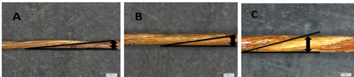
Figure 21 - Microscopic view of Symmetric Hybrid Cords at 250 tpm: ARA220x1+PET238x1 (A), ARA550x1+PET550x1 (B), ARA1100x1+PET1100x1 (C)
