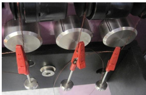
Figure 2 - Established pre-tension (minimum 10 cN)
