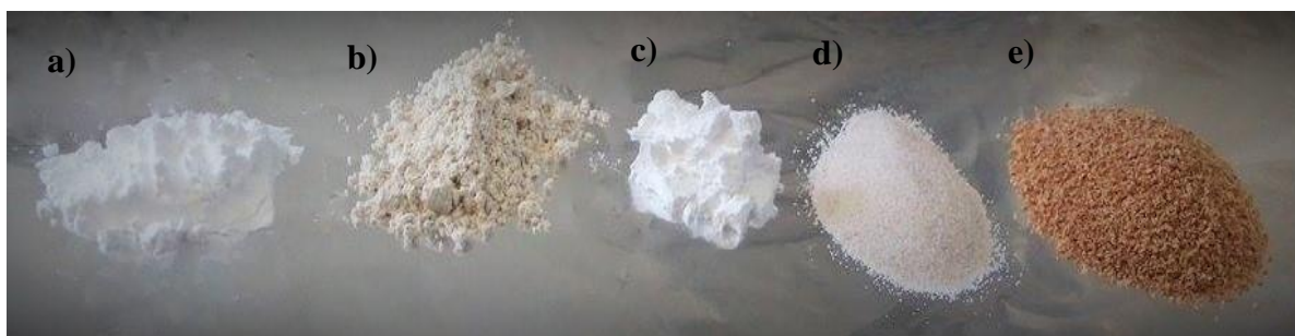
Figure 4 - Microparticles cores studied: a) calcium carbonate, b) kaolin, c) silica, d) sea sand and e) cork.
