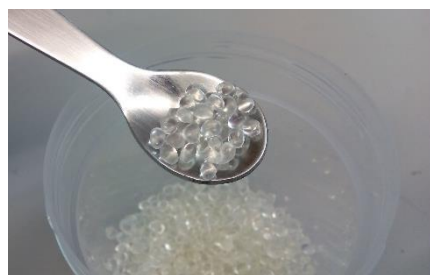
Figure 5. Tecothane® thermoplastic polyurethane (TPU) pellets.
