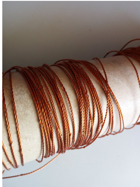
Figure 4.20: Twisted copper cable
