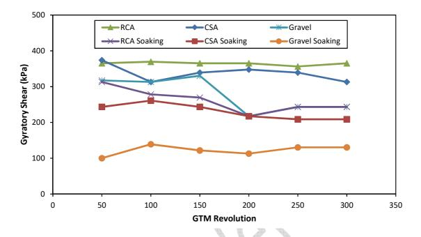
Figure 3 - Evolution of gyratory shear with GMT revolutions for different aggregates (adpated from Park, 2003).
