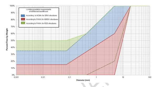
Figure 1 - Particle sizes recommended by FHWA (2010( and NCMA (2010).
