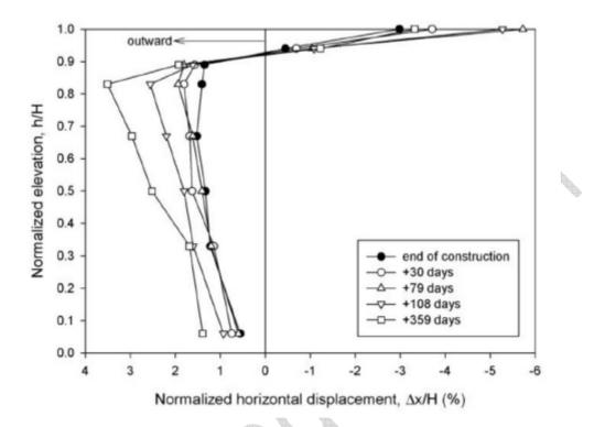
Figure 5 – Normalized horizontal displacements of the wall face recorded by Santos
