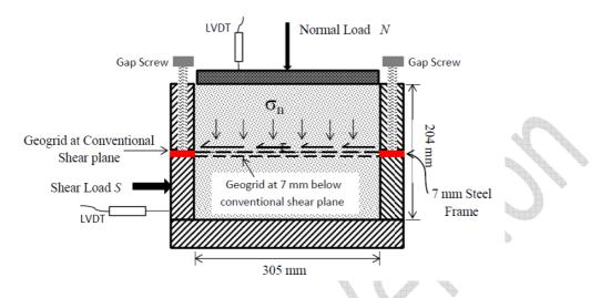
Figure 6 – Modified lower direct shear box with steel frame (Arulrajah et al., 2013b).
