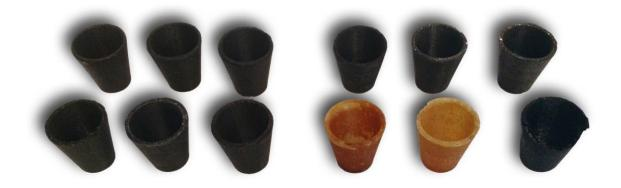
Figure 36 - Experiments with PLA/coffee on a silicone mould.
