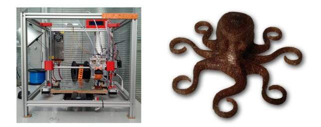
Figure 20 - 3D Printer, property of FEUP (left). 3D printed octopus using 3Dom coffee filament (right).
