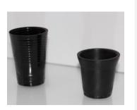
Finally, the combinations were deposited in rudimentary moulds and left to dry for 24 hours.
