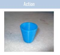
Before the first experiment with PLA, an object (cup) was created in Solidworks (CAD programme) and converted to STL format. It was then printed by method of FDM on one of FEUP's printers. The printer is a RepRap, developed at one of FEUP's laboratories and the filament is a 1.75 mm blue PLA, from 3D lnk.
