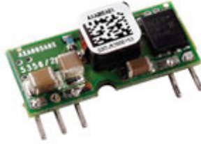
Figure 7.32: 12V to 15V DC-DC converter
