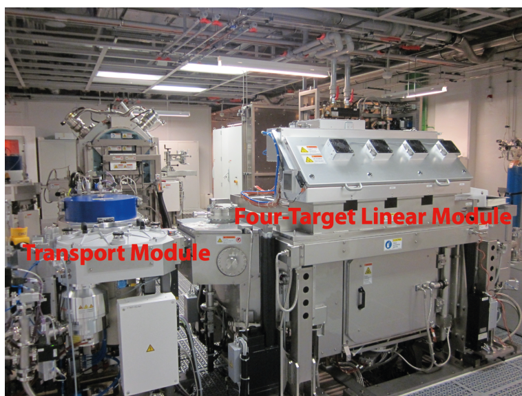
Figure 3.4: FTM sputtering tool used in this thesis. The cassette module is not shown because is similar to the one presented in Fig. 3.2.
