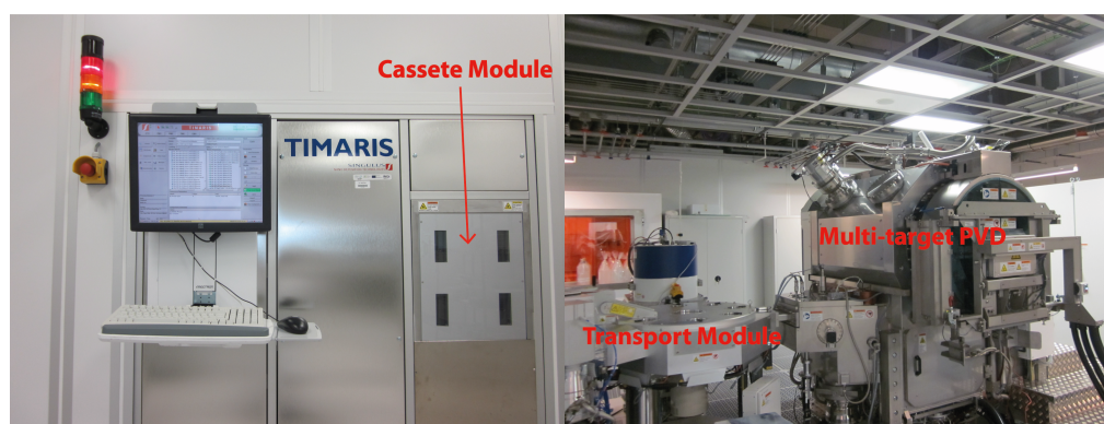
Figure 3.2: MTM sputtering tool used in this thesis. The images highlight the modules used for the stack depositions.
