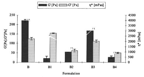
Figure 3. Storage modulus (G'), loss modulus (G"), and complex viscosity ( $\eta^*$ ) of the developed SLN and NLC formulations based on Compritol<sup>®</sup>888, after application of a frequency range between 0 and 10 Hz.
