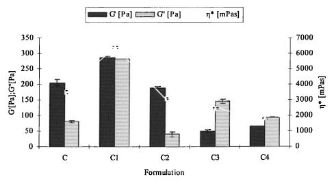
Figure 4. Storage modulus (G'), loss modulus (G"), and complex viscosity ( $\eta^*$ ) of the developed SLN and NLC formulations based on stearyl alcohol, after application of a frequency range between 0 and 10 Hz.
