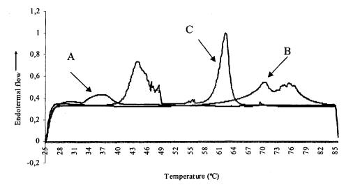
Figure 1. DSC curves of the developed SLN formulations (A, B, and C) recorded seven days after sample production.
