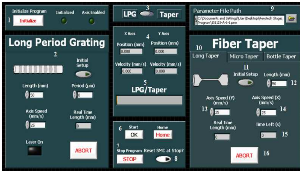
Fig A.1 - Front panel of the LabVIEW routine responsible for setting the taper fabrication parameters.
