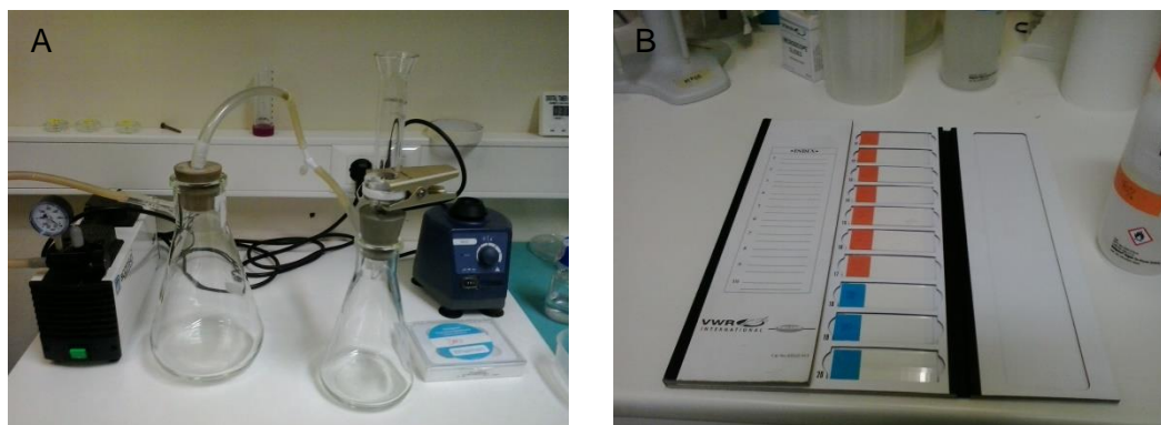
Fig. 15 - A: Vacuum filtration system; B: Sets of glass slides.
