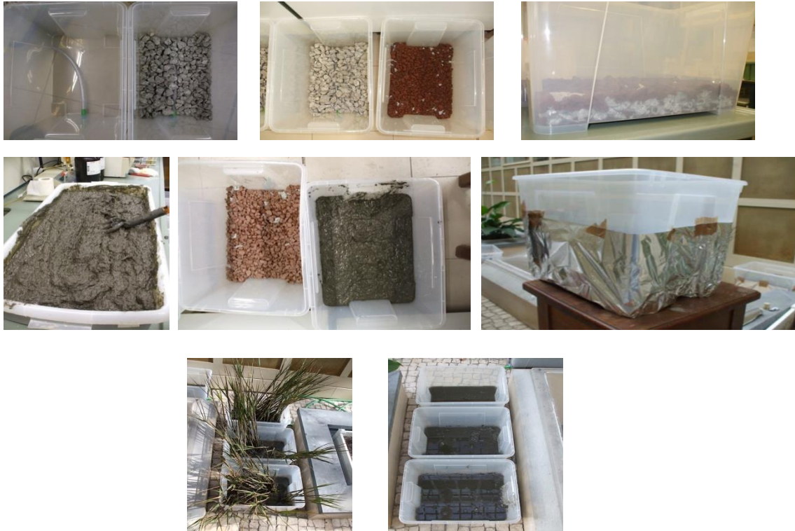
Fig. 14 - Constructed wetlands – microcosms setup ( Carvalho, 2012).
