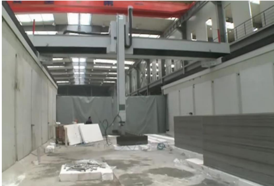
Figure 5.37 – 3D Printer by Win Sun [3]
