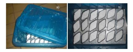
Fig. 7.1 - Experimental setup used to: (a) hold moisture absorber and of (b) the plastic trays used to hold each mixture.
