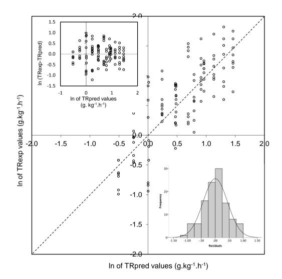
Fig. 6.4 - Relationship between transformed -natural logarithm- experimental (TRexp) and predicted (TRpred) transpiration rates, following Equation 6.4. Enclosed figures represent the residuals versus predicted values (top corner) and the frequency distribution of residuals with the solid line representing the expected normal distribution (bottom corner).
