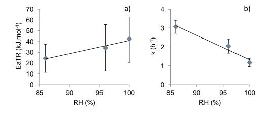
Fig. 6.3 – Effect of RH of the storage environment on the parameters of the Arrhenius model, (a) Ea<sub>TR</sub> (kJ.mol<sup>-1</sup>), and (b) k (h<sup>-1</sup>). The symbols represent the estimates of the individual model parameters, the bars represent the 95 % asymptotic confidence intervals and the lines represent the fit of the model (Eq. 6.2 and 6.3, respectively).
