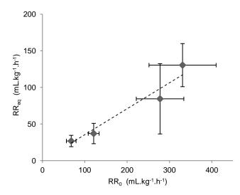
Fig. 4.4 - Relationship between individual parameter estimates of the initial respiration rate ( $RR_0$ ) and respiration rate at equilibrium ( $RR_{eq}$ ) at each temperatures used for model fitting (2, 6, 14 and 18 °C). Bars represent the asymptotic 95 % individual confidence intervals. Dotted line represents the linear fit between  $RR_0$  and  $RR_{eq}$  ( $R^2$ =0.940).
