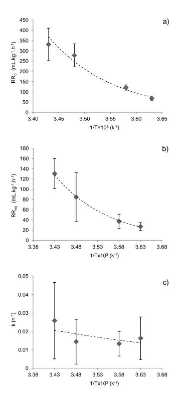
Fig. 4.3 - Dependence on temperature of the first order decay model parameters: a)  $RR_{0, ref}$  (mL.kg<sup>-1</sup>.h<sup>-1</sup>); b)  $RR_{eq, ref}$  (mL.kg<sup>-1</sup>.h<sup>-1</sup>) and c)  $k_{ref}$  (h<sup>-1</sup>). The dots represent the individual estimates and the bars represent the asymptotic 95 % confidence intervals (Cunha *et al.*, 2006) and the lines represent the fit of the model, according with Eqs. 4.4, 4.5 and 4.6, respectively.
