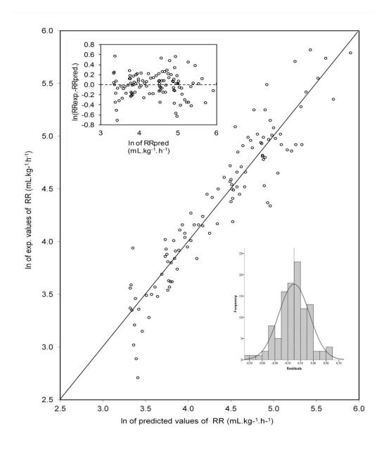
Fig. 4.6 - Relationship between experimental and predicted  $O_2$  consumption rates using the first decay model and assuming an Arrhenius type dependence of the model parameters on temperature (global model – Eq. 4.9). Enclosed figures represent the residual versus predicted values (top corner) and the frequency distribution of residuals, with — representing the expected normal distribution (bottom corner).
