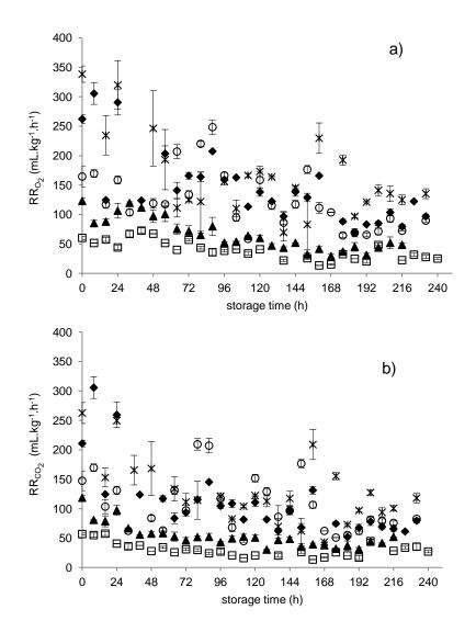
Fig. 4.1 - Evolution of a)  $RR_{O_2}$  and b)  $RR_{CO_2}$  (mL.kg<sup>-1</sup>.h<sup>-1</sup>) of oyster mushrooms stored at various constant temperatures under ambient air. Symbols represent the mean of 3 replicates and bars represent the standard error of the mean ( $\square$ - 2 °C;  $\blacktriangle$ - 6 °C;  $\circ$ -10 °C;  $\blacklozenge$ -14 °C;  $\star$ - 18 °C).
