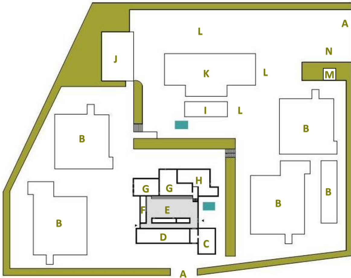
Figure 7. Architectural plan of the school complex. A – Entrance; B – Classroom block; C – Administration and secretary block; D – Teachers’ room; E – Recreation room; F – Cafeteria; G – Canteen; H – Library; I – Study room; J – Multipurpose rooms; K – Gymnasium; L – Sports ground; M – Storage unit; N – Parking lot
