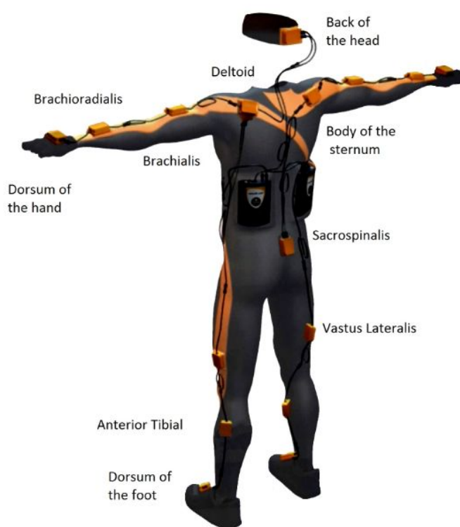
Figure 20. Positioning of inertial sensor modules.
