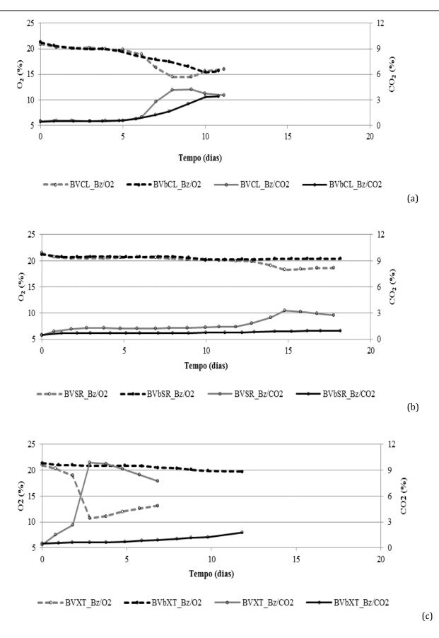
Figure 2. Time evolution of oxygen (O<sub>2</sub>) and carbon dioxide (CO<sub>2</sub>) in gas phase of remediation tests performed in: (a) limestone; (b) granite and (c) schist. Legends of the graphics (tests designations) are in accordance with Table 1.
