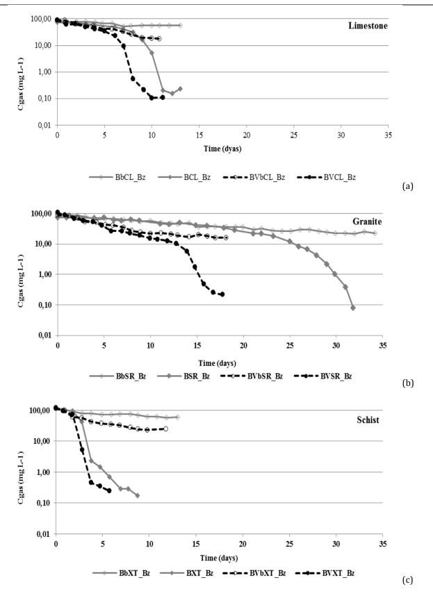
Figure 1. Time evolution of benzene concentration in gas phase (Cgas) from remediation tests performed in: (a) limestone; (b) granite and (c) schist. Legends of the graphics (tests designations) are in accordance with Table 1.
