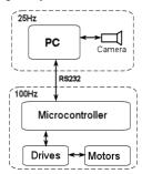
Figure 3: Robot's control and communication structure.
