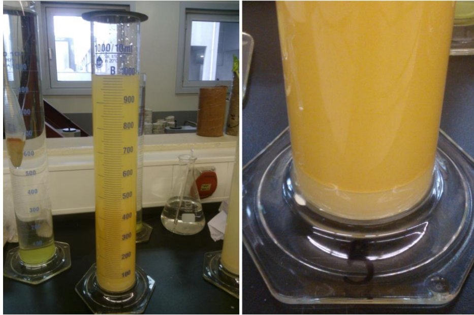
Figure 3.8 – Beaker used for specific gravity determination (left), detail on deposited particles after 24h (right)
