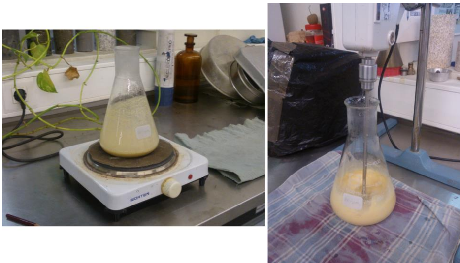
Figure 3.7 – Heating of soil sample with sodium hexametaphosphate (left), mixing of heated sample with a particle mixer (right)
