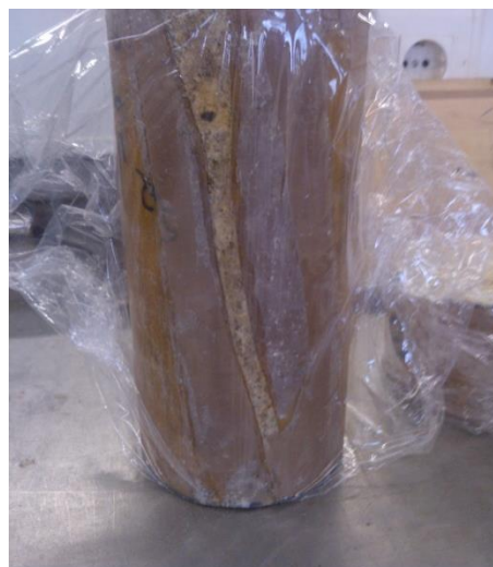
Figure 3.3 – Detailed view of the sampling liner crack
