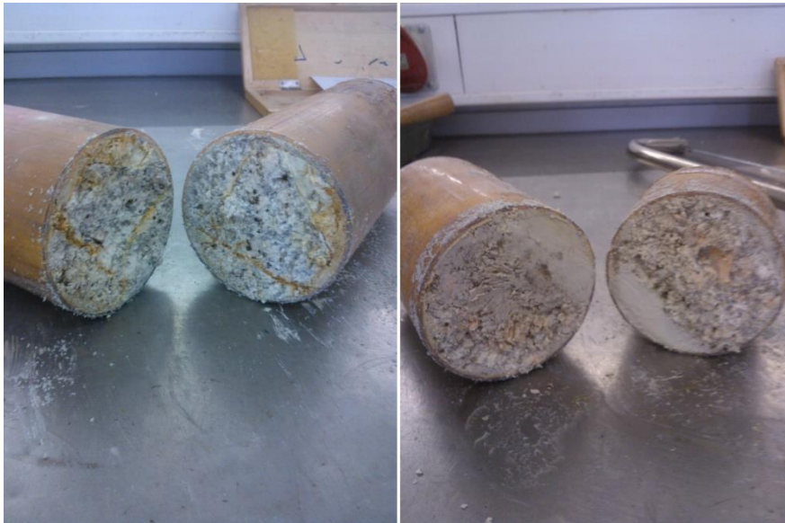
Figure 3.4 – Sawed surfaces: surface irregularity (left) and presence of finer mass (right)
