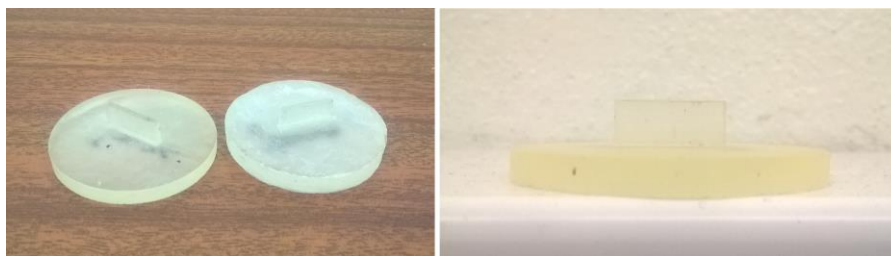
Figure 5.1 – Negatives used for bender element installation
