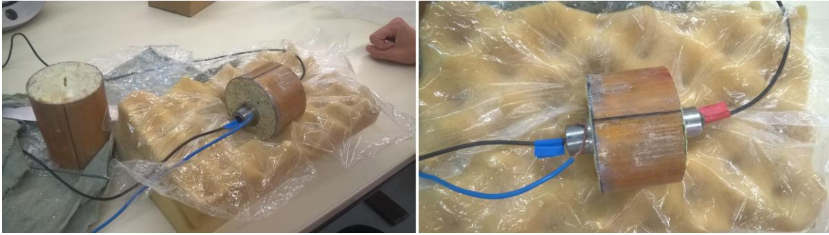
Figure 4.22 – New bender element test methodology
