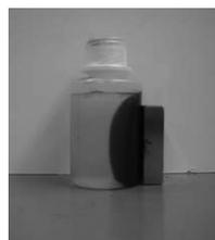
Fig. 1 – Magnetic response of  $Fe_3O_4$  colloidal suspension in the presence of a magnet.
