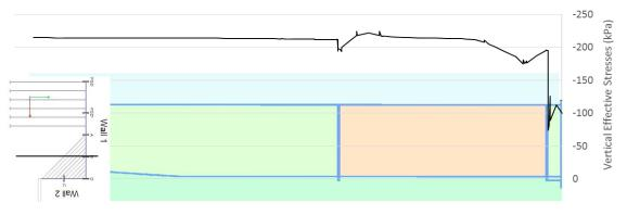
Figure 5.32 - Effective vertical stresses at depth -11m, in a cross section at x=19
