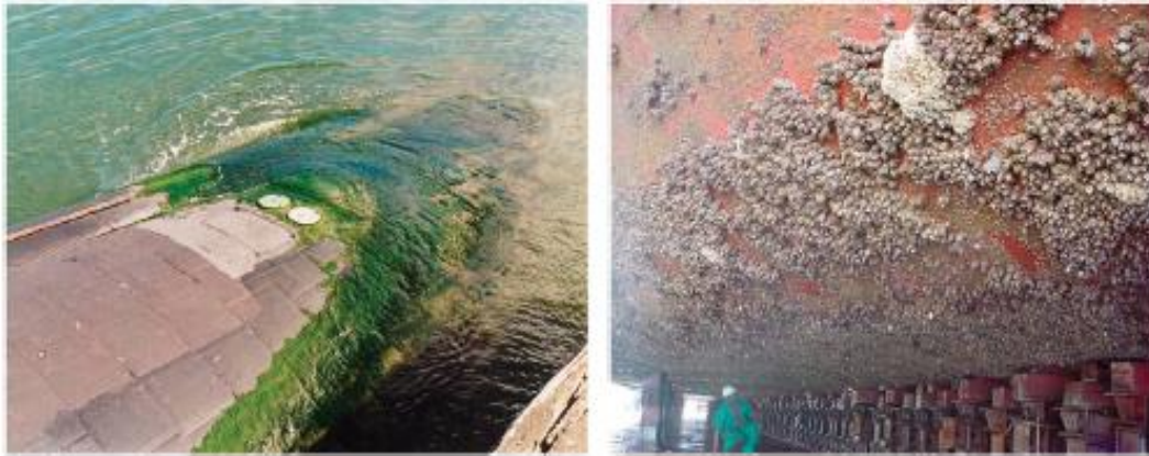
Figure 1 – Shipp hulls with biofouling (adapted in Callow et al. , 2011)
