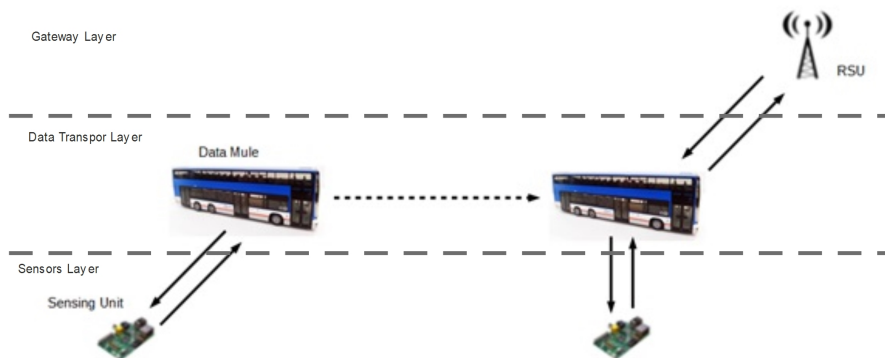
Figure 3.3: Three layers architecture of data mulling.
