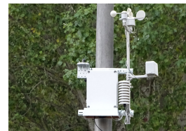
Fig. 1. Sensing device deployed in R. Damião de Góis, Porto, Portugal. UrbanSense sensing devices are processing devices (Raspberry Pi) equipped with environmental sensors (wind direction and speed, rain, solar radiation, luminosity, humidity, temperature, noise) and a IEEE 802.11b/g/n interface.
