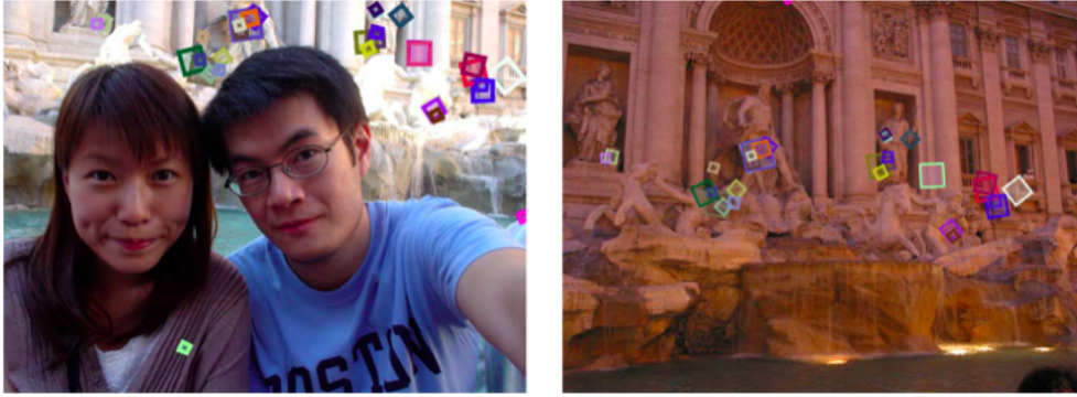
Figure 2.28: Example of a SIFT descriptor matching found in two different images of the same sight. Extracted from [78].
