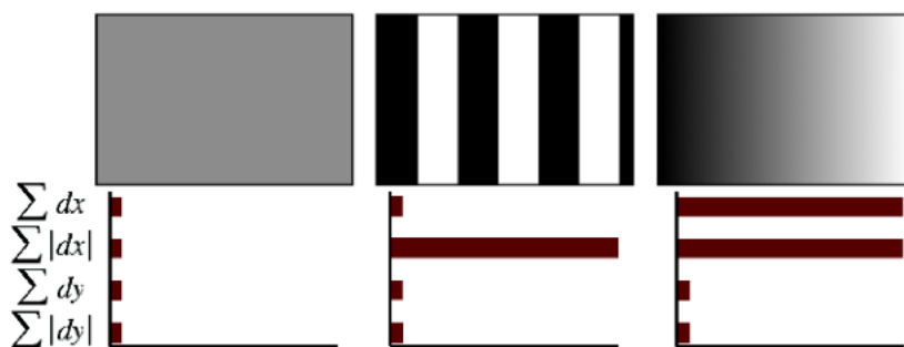
Figure 2.30: The descriptor entries of a sub-region represent the nature of the underlying intensity pattern. Left: In case of a homogeneous region, all values are relatively low. Middle: In presence of frequencies in x direction, the value of |dx| is high, but all others remain low. If the intensity is gradually increasing in x direction, both values |dx| and dx are high. Extracted from [81].
