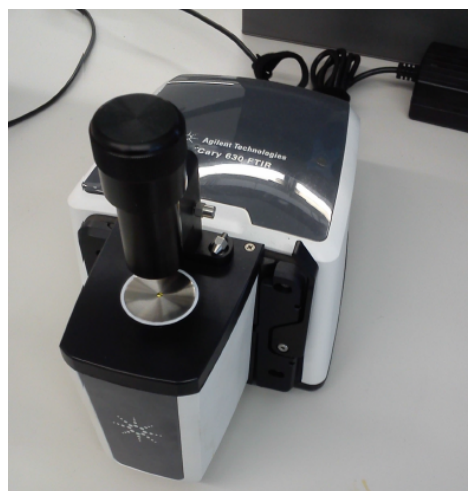
Figure 3.6.: FTIR working principle and Agilent Cary 630
