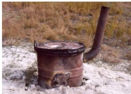
Figure 2.1 – Incinerator used to treat HCW in a developing country (source: Diaz et al., 2005).
