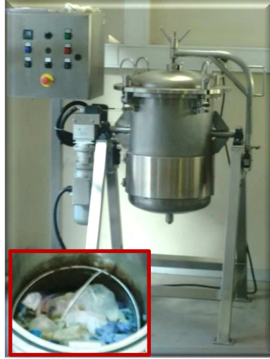
Figure 8.1– Pilot reactor and real infectious HCW used in the alkaline hydrolysis tests.
