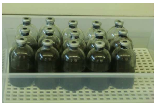
Figure A.3.1 – The samples, blank and controls vessels used in anaerobic tests.
