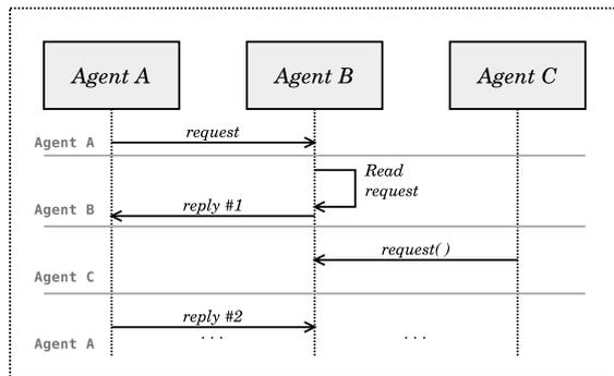
Figure 8: Asynchronous communication.
