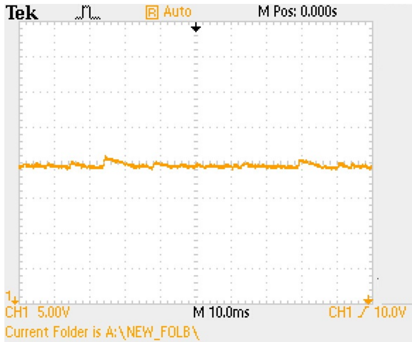
Figure 3.19: Output voltage of the driver.
