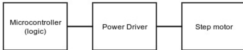
Figure 2.38: Stepper motor driver block diagram.
