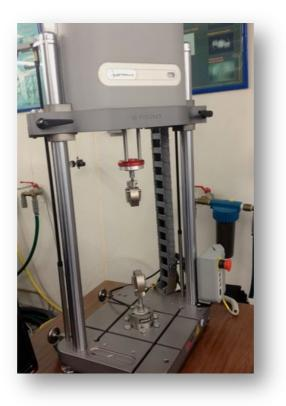
Fig. 4 - Instron ElectroPuls E1000 machine.
