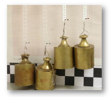
Fig. 9 – Photograph after 18 days (432hours) of constant load tension application. No change in the initial position of the marks occurred.
