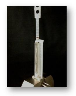
Fig. 5 – Specimen from Ceosa<sup>®</sup> during tensile test; view of the disengagement of the coil spring from the plastic strap.
