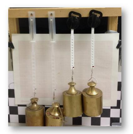
Fig. 7 – Customized support structure for the constant load tension test.
