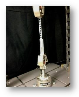
Fig. 6 – View of specimen C4 from Ceosa<sup>®</sup> during the short-term fatigue test in the *Instron* machine.
