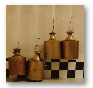
Fig. 8 – View of specimens C5, C6, O5 and O6 with 9,8N calibrated masses in suspension.
