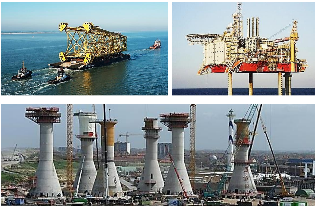
Figure 3.1. – Jacket platform (top left) [1]; Jackup (top right) [2]; Gravity foundations (bottom) [1]
