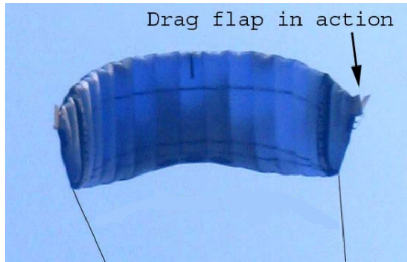
Figure 2.8: Drag flap control mechanism [7].
