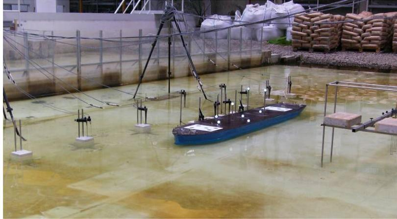
Fig. 3 The physical model in the wave tank.
