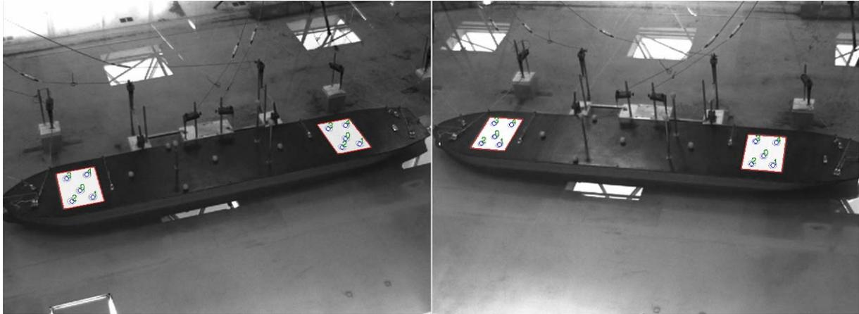
Fig. 8 Stereo images from the developed system of the physical model with dice-like markers being processed.
