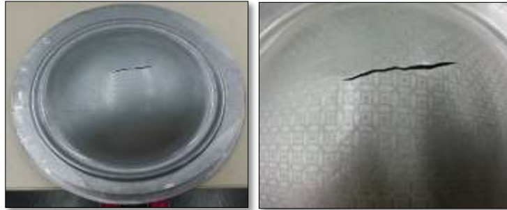
Figure 3.6: Final part of Hydraulic Bulge Test
