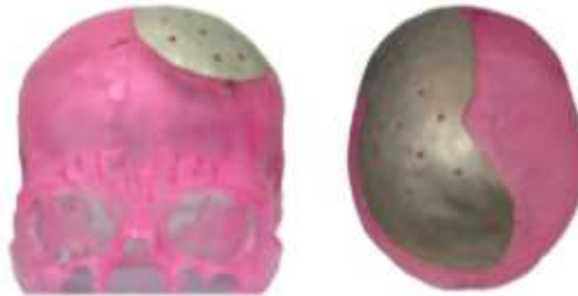
Figure 2.17: Cranial plate for medical application [27]
