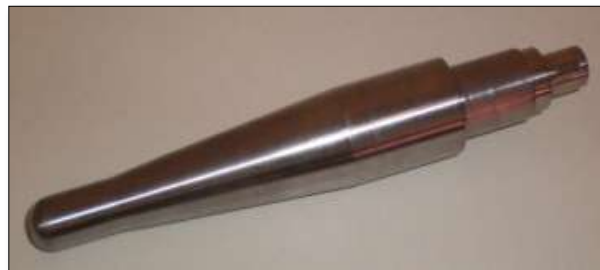
Figure 3.16: Hemispherical forming tool with 12 diameters tip [1]
