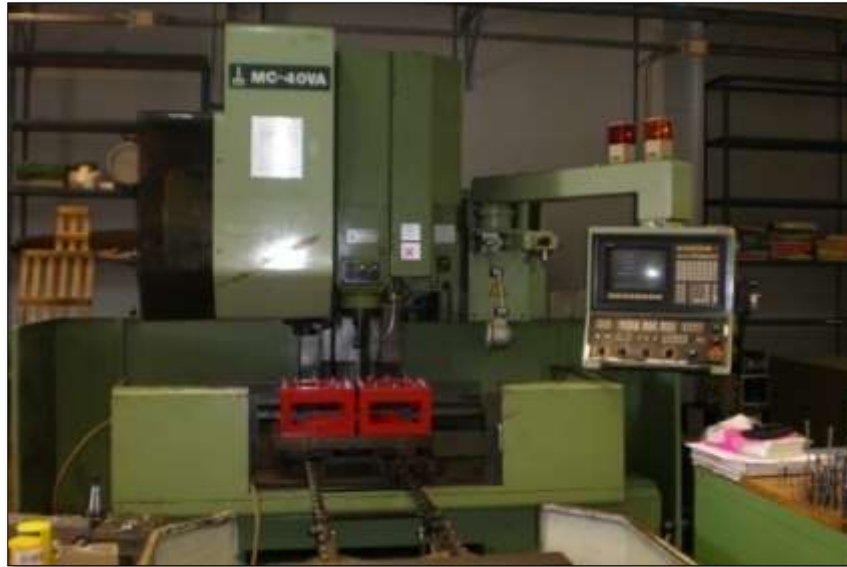
Figure 3.18: OKUMA MC-40VA CNC 3 axis vertical milling machine at Faculty of Mechanical Engineering workshop [13]
