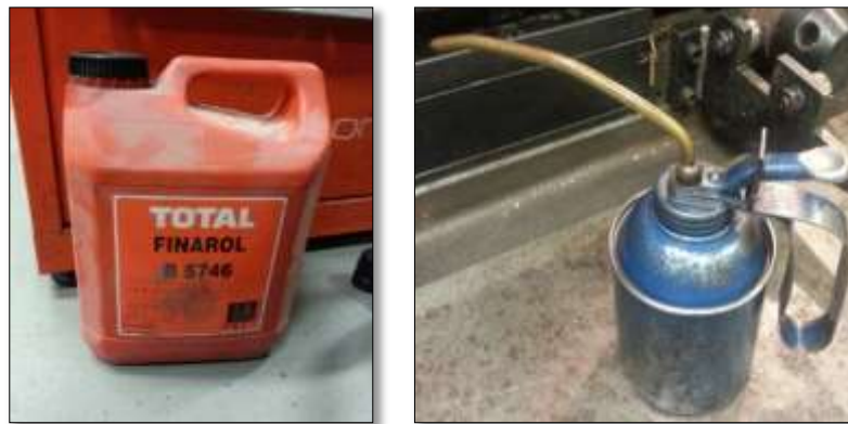
Figure 3.20: Lubricant for ISF manufacturing
