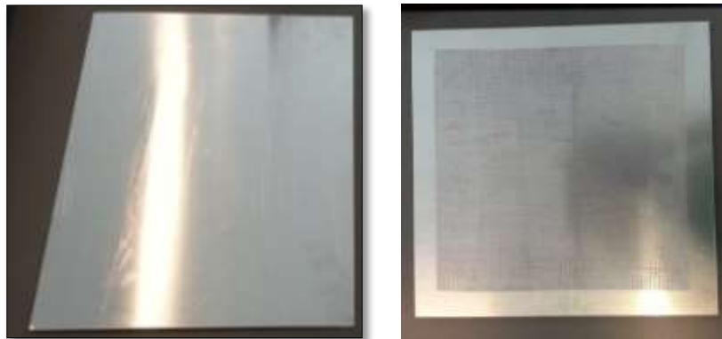
Figure 3.12: 250 x 250 Aluminium 1050-H111 sheet for SIF manufacturing
