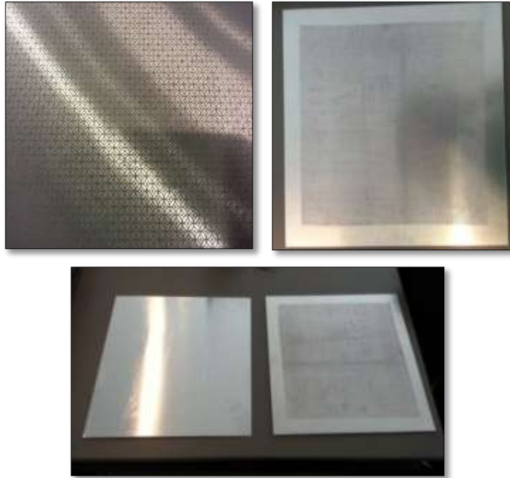
Figure 3.13: Sheet metal with grid marks
