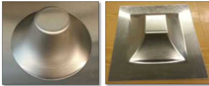
Figure 3.38: SPIF finished part
