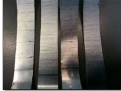
b. Scratch mark on the sheet
