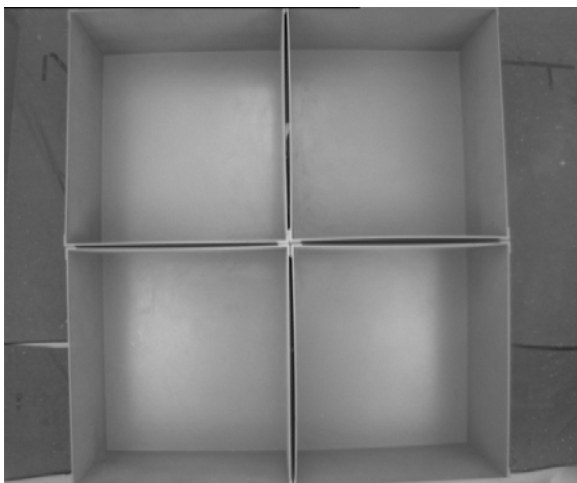
Fig 2. Open Field. made of four grey plastic boxes of 78 x 78 x 45 cm and was positioned in a testing room with diffuse lighting. Four subjects (one per box) can be tracked at the same time. General activity is recorded and measured in terms of distance travelled in the box.
