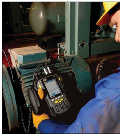
A technician uses a predictive maintenance handheld tool to perform an asset conformance check with overall and frequency-based vibration readings.
