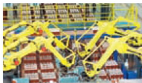
This ASI unloader was designed to handle 40,000 modular brick per hour.
