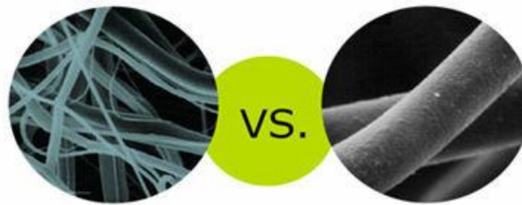
Figura 4 - Microfibras Thinsulate™ vs. Fibras de poliéster convencionais (3M®, 2009)
