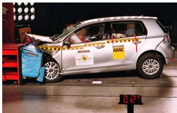
Figura 21 – Teste experimental impacto Frontal (Euro NCAP, 2010).
