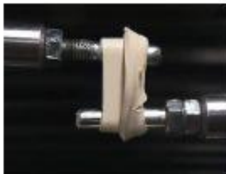
Figure 16 - Radial tear strength tool performed with INSTRON equipment.
