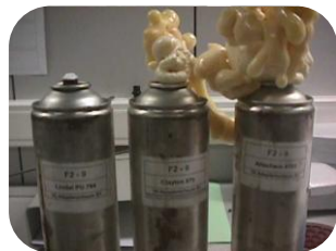
Picture comparing the three tilting valves for the foam 2, week 20: The stem of the can on the left was broken due to the hardening of the grommet, while the two valves on the right did not close properly once they were activated.
