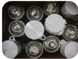
Example of valves arrived in bad state
