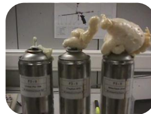
Picture comparing the three tilting valves for the foam 3, week 20: There is foam releasing between the stem and the grommet of the can on the left, while the two valves on the right did not close properly once they were activated.
