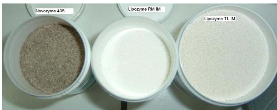
**Figure 2** – Different enzymes test in this work: Novozyme 435, Lipozyme RM IM and Lipozyme TL IM
