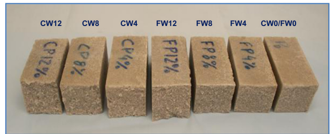
Fig. 3. Samples of broken PM test specimens after being tested in flexural (one sample of each CW and FW test series).
